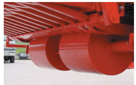
"Under head" roller supporting the harvesting head
