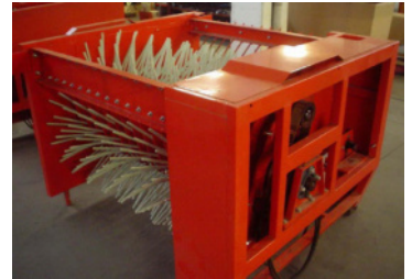
Complete vibrating rays equipment for plant separation
