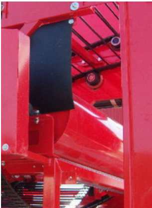
Rear roller on the transversal belt for the elimination of waste
